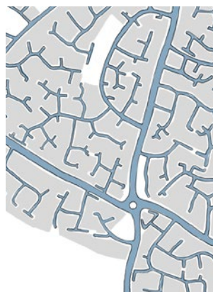
Figure 111: The differences between a disconnected and connected network of streets as illustrated in the National Model Design Code. Connected streets help to reduce walking distances and set a long-lasting framework for movement.
